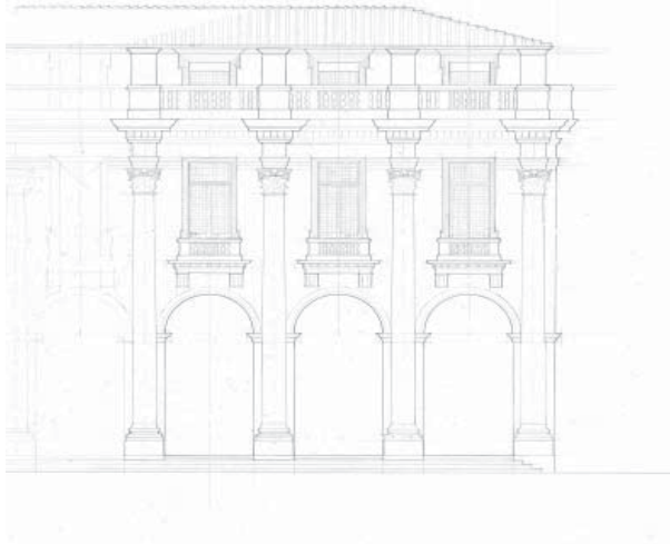
Fig. 1 Pencil on hot-press paper. Drawing of Palladio's Loggia del Capitaniato. Student work by Tim Hoefft. The drawing was completed from site measurement, sketches and observations
